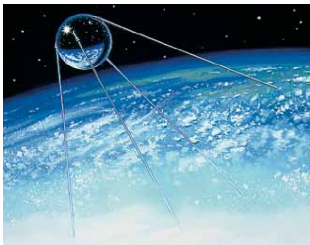
Fig 7 Sputnik 1 was the Earth's first artificial satellite. It was relatively small with a mass of 84 kg and a diameter of 53 cm. Its four aerials beamed back information about the temperature and density of the upper atmosphere.
