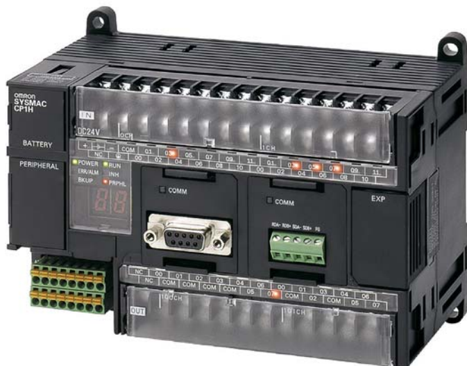
Figure 14-44 Omron PLC with Modbus-RTU network communication capabilities. Source: Photo courtesy Omron Industrial Automation, www.ia.omron.com .
