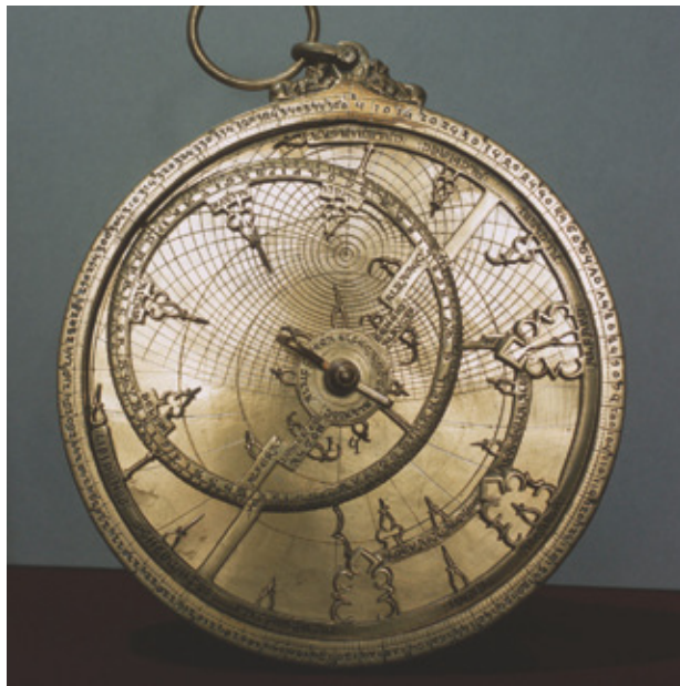
Source 3.57 An astrolabe was used to chart the movements of planets and stars.
