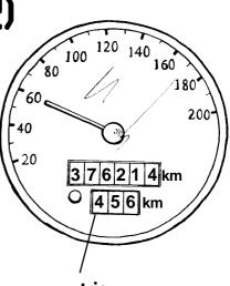
trip odometer (pressing the button will reset it to 0)
