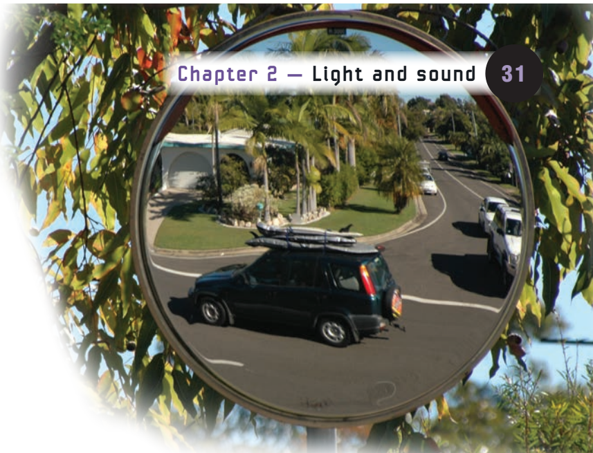
Fig 4 Convex mirrors are used on dangerous road intersections. Light rays from wide angles strike the mirror, giving a wider-angle image than would be seen using a plane mirror.
