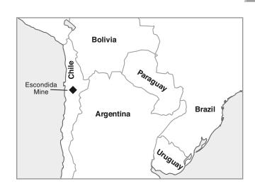
the country in the Atacama Desert. The largest copper mine in the world, Escondida, is located there. Over 900 000 tonnes of copper are mined each year from two giant pits in Escondida. About 4000 people work at the mine.
